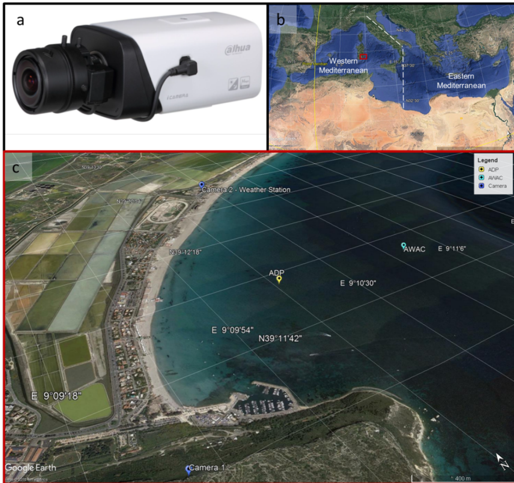
Figure 6.1 (a) Video-camera adopted for coastal video-monitoring station at Poetto beach. (b) Location of the study area in Western Mediterranean Sea, Cagliari Gulf, Sardinia, Italy. (c) 3D view of cameras, weather station, AWAC and ADP location during "Poetto" experiment, courtesy of Google Earth.
