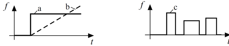
Figure 1.3: Time dependency of faults: abrupt (a); incipient (b); intermittent (c)
