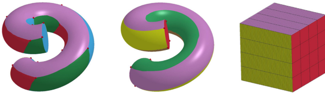
Figure 1.13: Pipeline recap (from [HZL17]): the segmentation using the first step, the skeleton-based segmentation and the final polycube.
