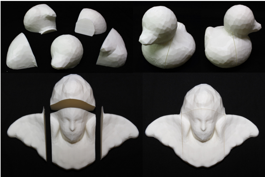
Figure 6.10: The models of Duck and Angel. On the top left the five printed parts of the Duck, and on the top right two views of the assembled model. On the bottom left the four parts of the Angel, and on the bottom right the assembled model.
