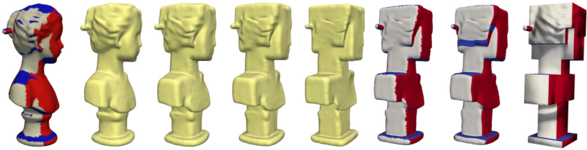
Figure 1.6: Pipeline recap (from [GSZ11]): from the original model to the polycube, after the deformation iterations.
