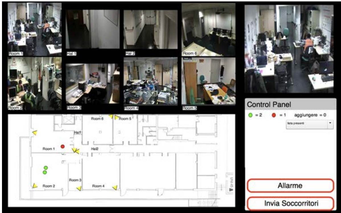
Figure 37 The Condition 3 simulator's interface layout. Inside the control panel is possible to view the number of workers and rescuers present in the lab. The green and red dots on the map represent the location of individuals.
