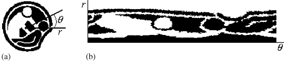
Figure 2.7: (a) An original shape in polar space. (b) polar-raster sampled image plotted in Cartesian space.
