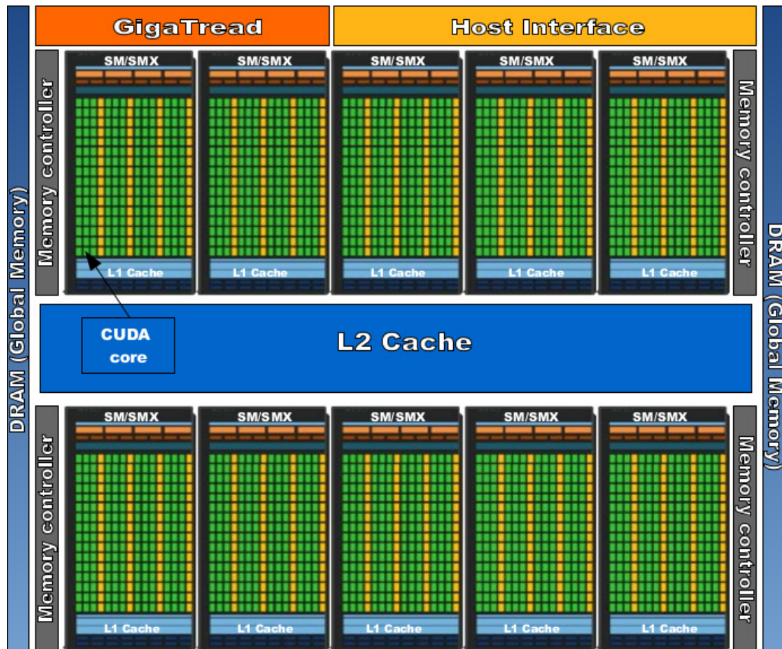
Figure 2.3: GPU Architecture. The NVIDIA GPU is a many-core processor equipped with hundreds of cores able to simultaneously handle thousands of threads.
