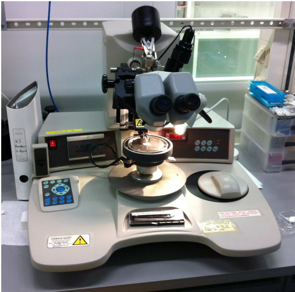
Figure 4.27: Wire bonding machine: Kulicke and Soffa 4526 .
