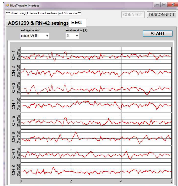
(b) On-line plotting window in a \mu V amplitude scale and with a 6s temporal window
