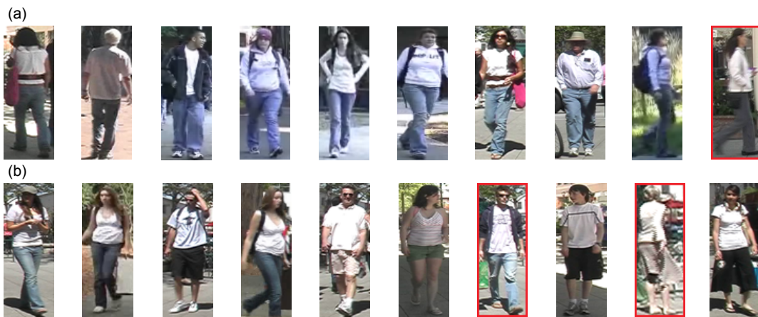
Figure 4.7: The top ten images retrieved by MCD_3 , for the queries “white shirt and blue trousers” (a) and “white shirt and short sleeves” (b). The images are sorted from left to right, for decreasing values of the score computed using a fuzzy logic approach, as the minimum of the scores produced by the detectors of the embedded basic queries. Non-relevant images are highlighted in red.
