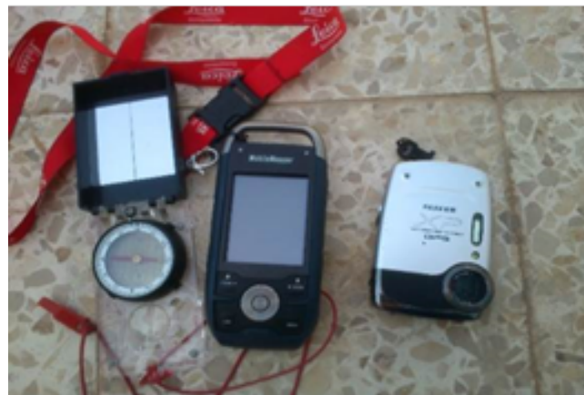
Figure 32. Instruments used for ground truth data collection: GPS incorporated Photo Camera, compass, GPS
