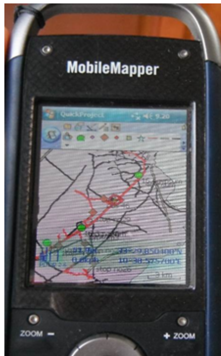
Figure 33. GIS software ArcPad installed on Mobile Mapper GPS; the visible loaded layers are: study area limit, GPS tracklog, doubt points, routes and toponyms, on site collected ground truth points (with attributes)
