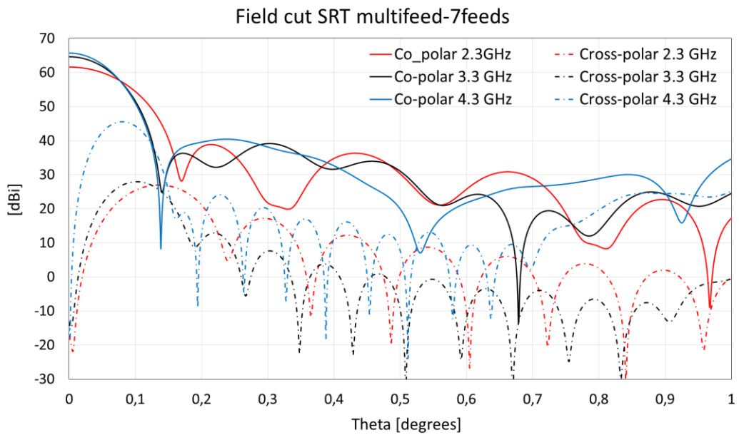
Fig. 4.46: Radiation pattern of the SRT with the multifeed system (7 feeds).
