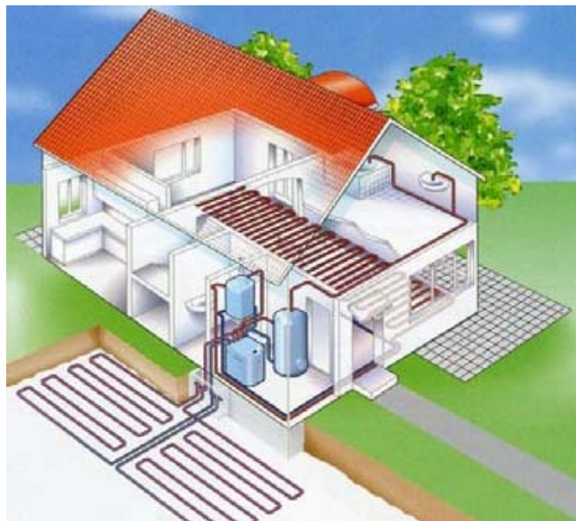
Figure 1.18 - Schematic representation of horizontal probes.
