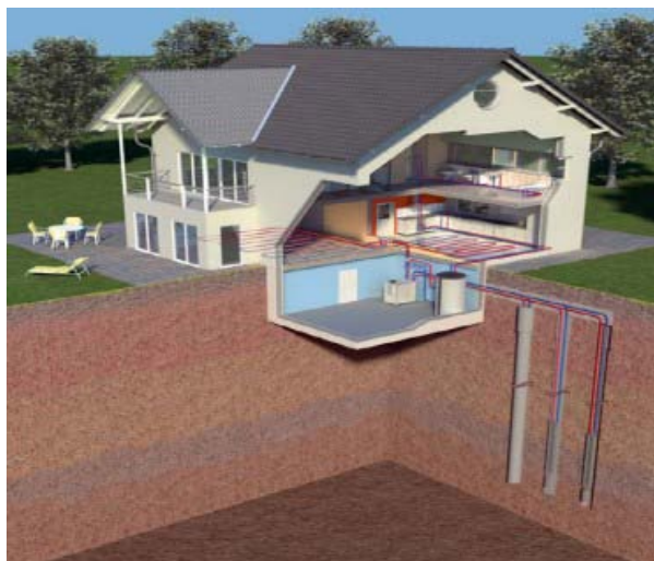
Figure 1.7 - Schematization of the vertical geothermal probes (from www.tekneco.it ).
