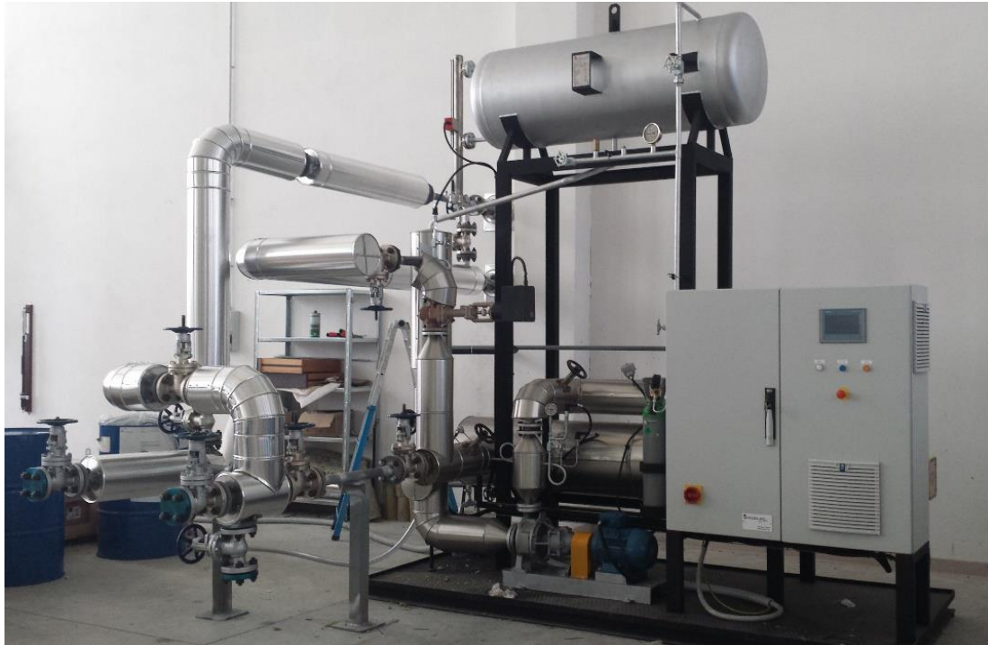
Fig. 5.4 - Skid of the test rig
