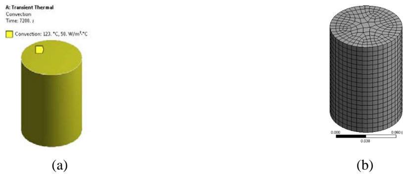
Fig. 30- (a) Convective boundary condition applied on the surfaces of model (b) Shows the 3D model meshed
