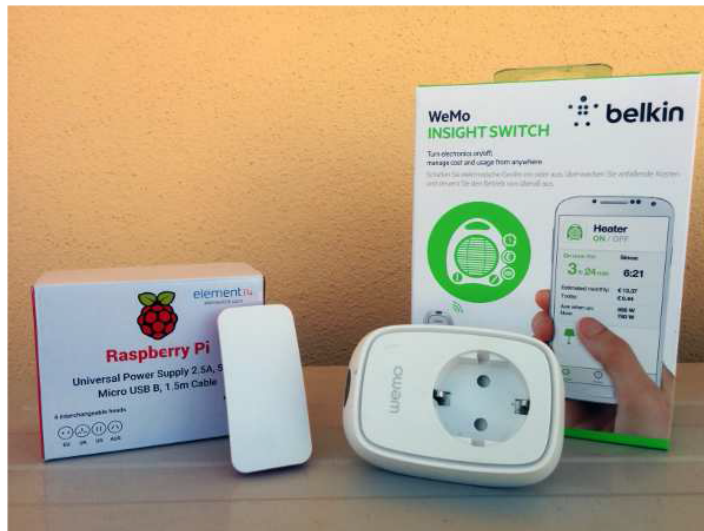
Figure 6.16: A Raspberry Pi-0-W and a smart socket
