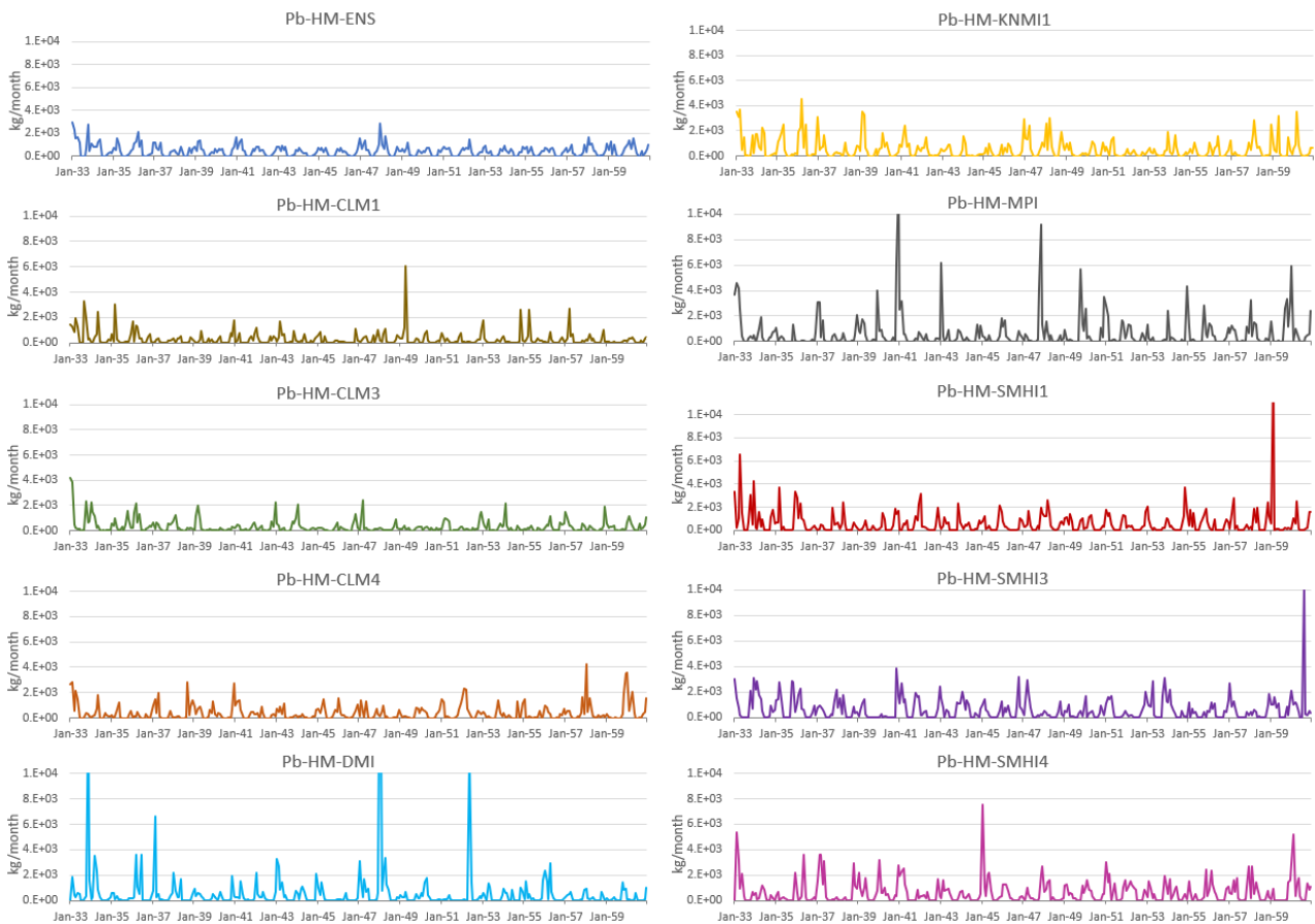
Figure 84 - Pb total yearly load simulated in Rio San Giorgio's outlet using different climate forcing models by SWAT-HM
