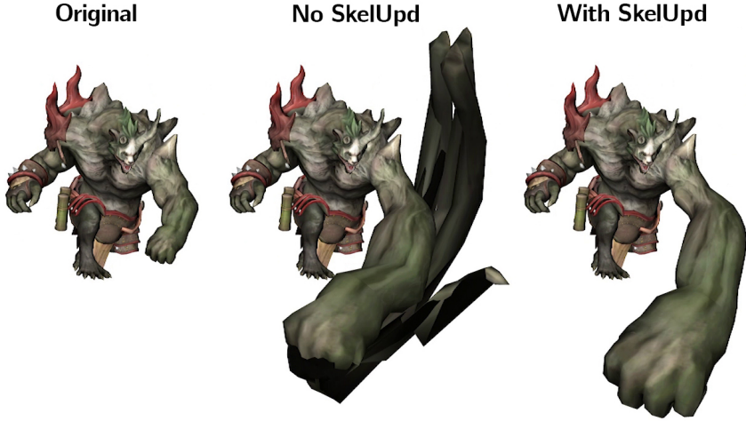
Figure 3.7: A comparison between the original skeleton deformation (left), skeleton deformation with cage edits plus skeleton updater disabled (middle), skeleton deformation with cage edits and skeleton updater enabled (right).
