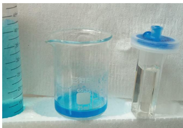
Figure 52.9. Copper-sulfate solution on the left, blue precipitation by adding drops of aqueous 1M KOH (middle) and after filtration by 0.22 \mu\text{m} syringe filter (right).
