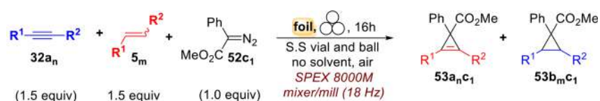
Scheme 46. Metal Foil-Catalyzed Cycloaddition of Unsaturated Hydrocarbons with Methyl Phenyl diazoacetate. Adapted with Permission from Ref 116. Copyright 2018 The Royal Society of Chemistry
