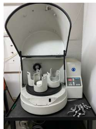
Figure 1. Fritsch-pulverisette 5, a planetary ball mill.
