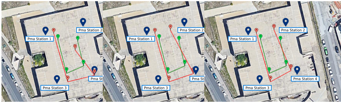
Figure 3.4: Ground truth trajectory (green) and trajectory (red) computed with RSSI-based algorithm.
