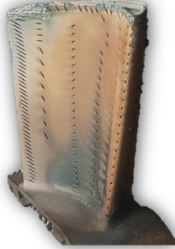
Figure 1.4: Damaged high pressure turbine blade
