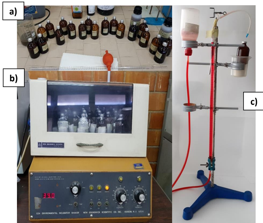
Figure S.21 – BMP tests: a) samples preparation, b) incubation, and c) biogas measurement.
