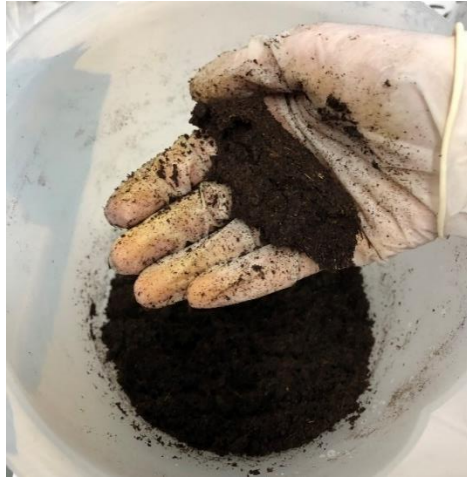
Figure S.9 – Fist method for the water content determination for the mixture preparation in germination tests.
