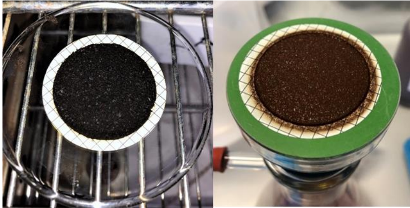
Figure S.6 – Solid residues (solid suspended) on acetate filter (0.45 \mu\text{m} ) after PW filtration.
