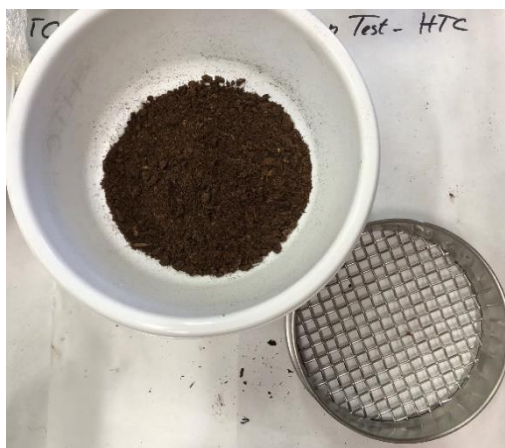
Figure S.8 – Sphagnum Peat after sieving (< 10 mm).
