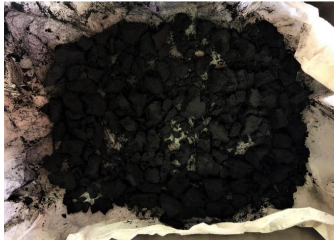
Figure S.4 – Wet hydrochar (from SCG) after separation through filter press.
