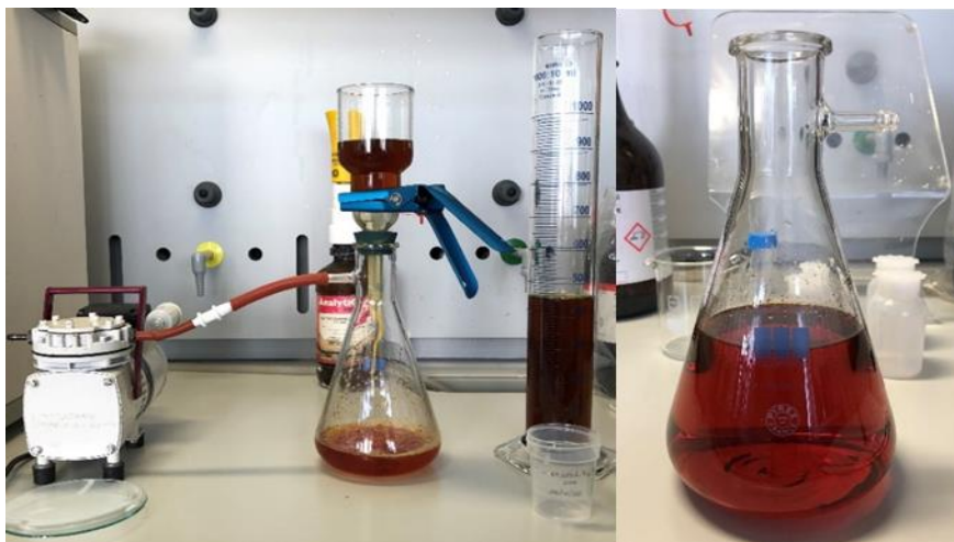
Figure S.5 – Vacuum filtration of PW and PW filtered.
