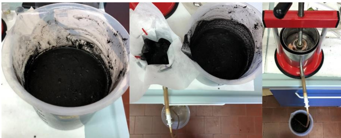
Figure S.11 – Washing phase for HC_220_1 with distilled water.
