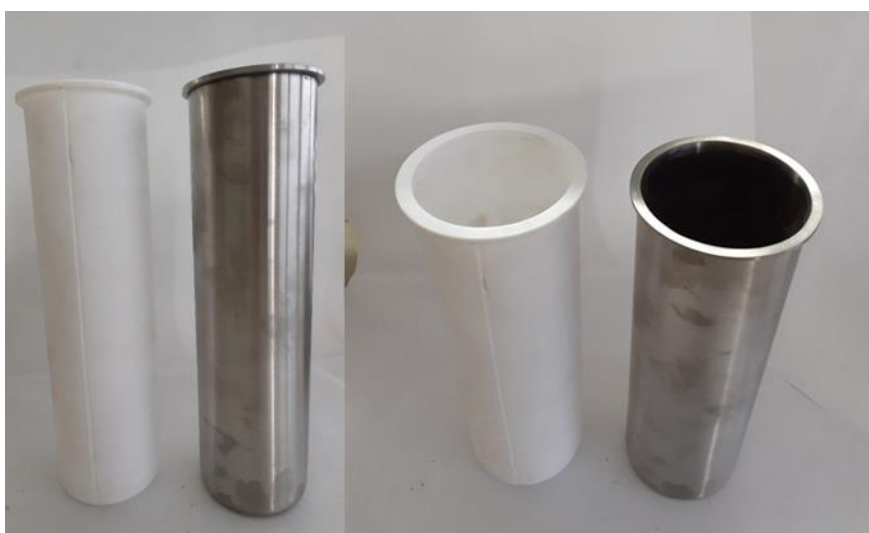
Figure S.2 – PTFE vessel and stainless-steel vessel.
