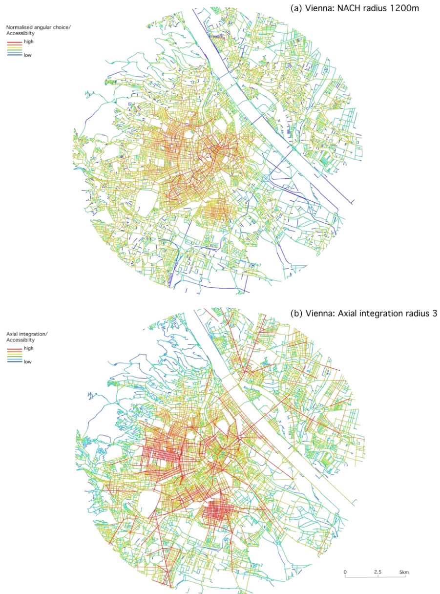
Figure 2. Local configurational analysis of Vienna's street network: (a) NACH radius 1200m, (b) Integration radius 3 (axial map credited to Sebastian Zeddel; model computed by the authors)
