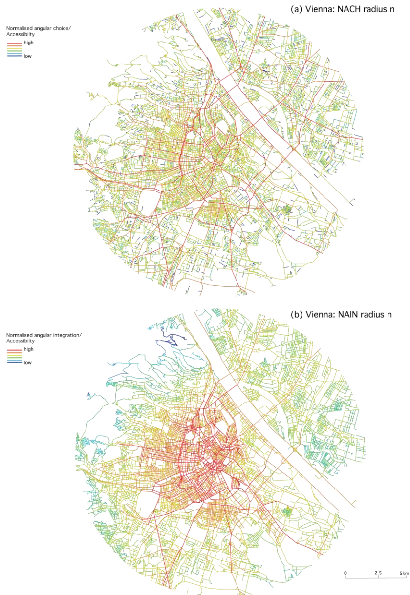
Figure 1. City-wide configurational analysis of Vienna's street network: (a) NACH radius n, (b) NAIN radius n [6] (p. 526), [12] (p.77)
