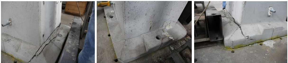
Figure 8. Collapse mechanism for different mixes: left RC0%, center RC30%, right RC50%
