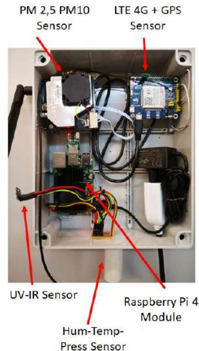
Fig. 7: Prototype of the environment monitoring sub-system.
