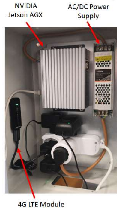
Fig. 6: Prototype of the mobility monitoring sub-system.
