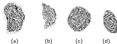
Figure 3: Examples of acquired PAs of ScreenSpooF in the wild data set. Green Bit: full (a); partial (b). DigitalPersona: full (c); partial (d).
