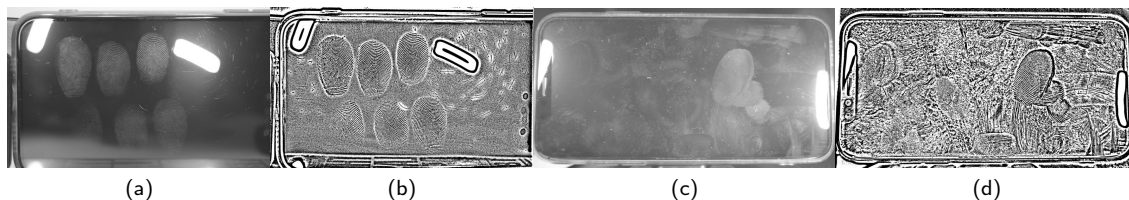
Figure 2: Differences between the first two steps of ScreenSpooF method using different acquisition protocols: in vitro acquisition (a) and binarization (b); in the wild acquisition (c) and binarization (d).
