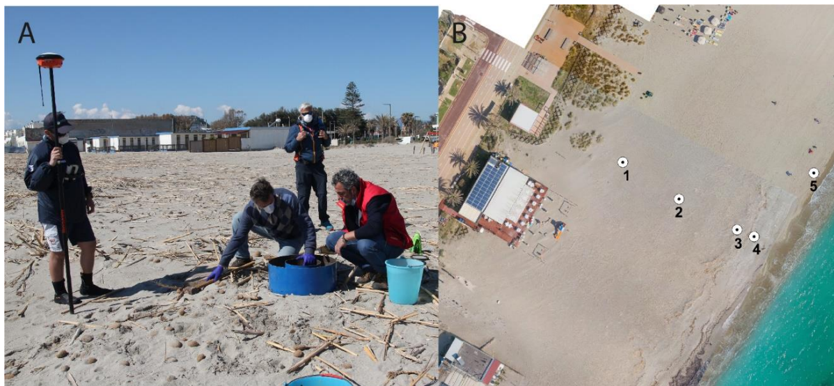
Figure 3.5 – Two drone images with location points of water infiltrometric tests, at Poetto beach.
