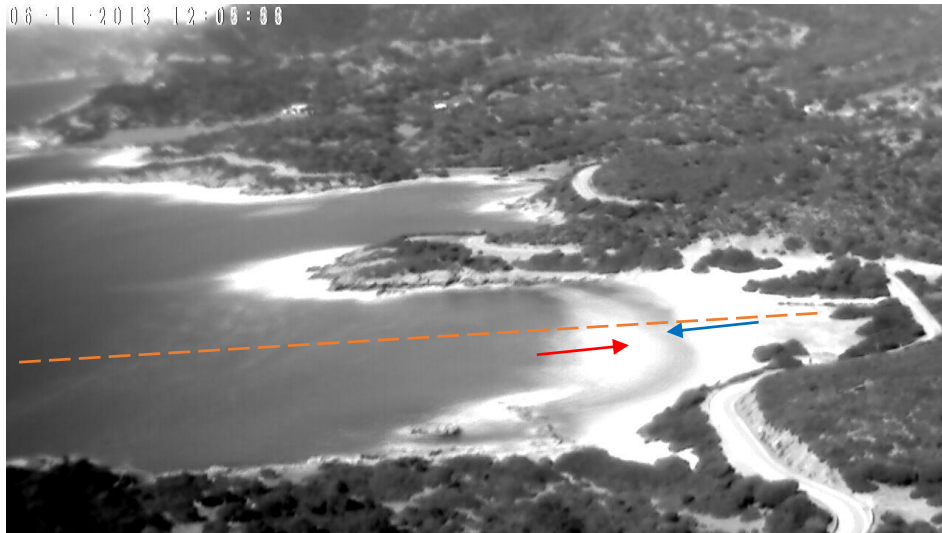
Figure 4.3 - Timex exposure of Piscinnì beach showing the morphology of the shoreface during a wave event. Red arrow shows the bar, blue arrow shows the trough and orange line represents the hypothetical transect.
