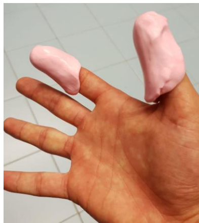
Figure 3.3: Creating a mold with silicone rubber (RTV).
