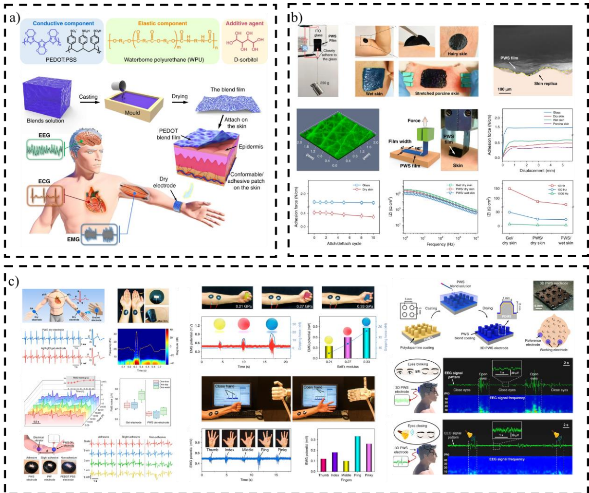
Figure 19 Zhang et al. [39]: fully organic dry, conformal, and self-adhesive electrodes for biopotential recording. a) fabrication process; b) conformability, adhesiveness, and contact impedance study; c) biopotential acquisitions: ECG, EMG, and EEG signals recording.
