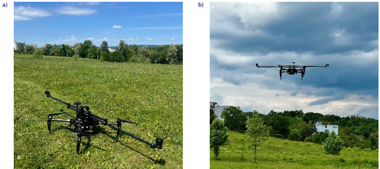
Figure 3. The DJI M100 UAS fitted with two Calypso anemometers: a – detailed view before the commencement of the flight, b – during performing the initial flight test
