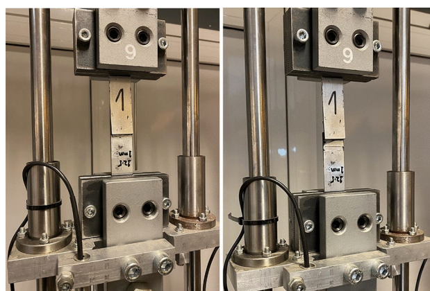
Figure 10. Creep test stand - the sample is subjected to a load of 3.0 kN (80% of failure load).
