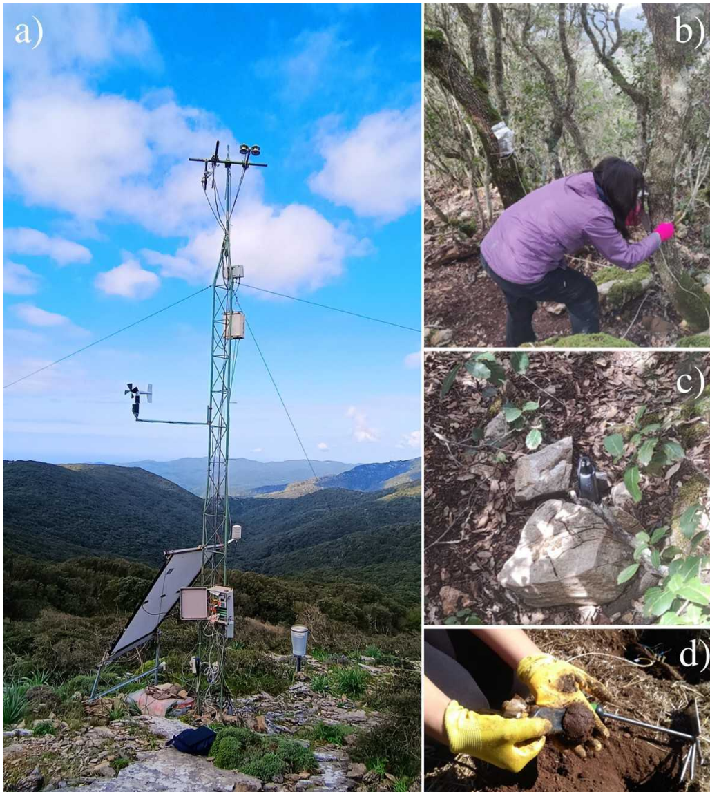
Figure 2.18: Marganai setup and equipment: a) micrometeorological tower, from the top to the bottom there are installed CSAT3B, LI-7500, NR-1 and the SI111 that measure canopy surface temperature. At about 5m height an bi-directional anemometer RMYoung 05103, and at 2m height the HygroVue from Campbell Sci., at about 5m from the tower it's installed the raingauge PMB2 CAE; b) Intallation of the sapflow sensor;c) \Delta T theta probe d) installation of the MPS2.
