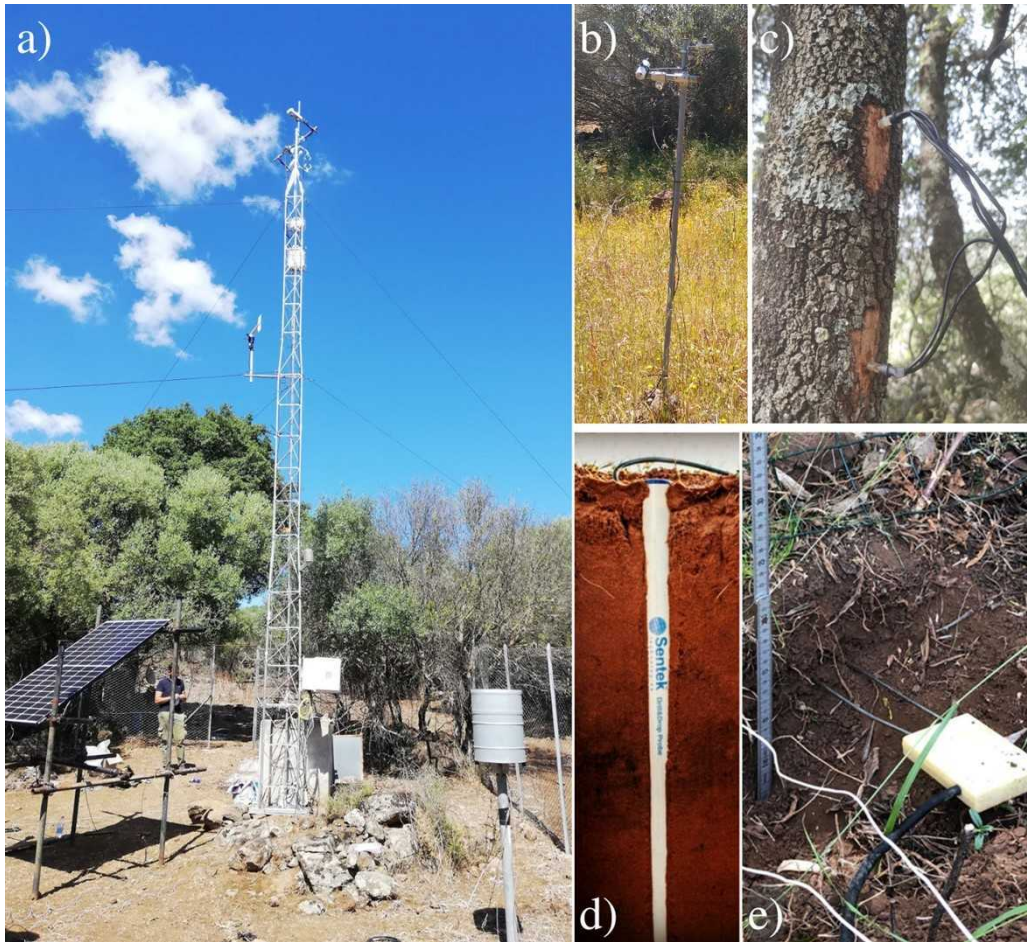
Figure 2.3: Orroli setup and equipment: a) micrometeorological tower, from the top to the bottom there are installed CSAT3B, LI-7500 and CNR-1, at about 7m height an bi-directional anemometer RMYoung 05103 and the SI111 that measure canopy surface temperature, at 2m height the HygroVue from Campbell Sci., at about 5m from the tower it's installed the raingauge PMB2 CAE; b) SI111 that measure grass/bare soil surface temperature and SQ-110; c) sapflow sensor; d) example of the installation of the Sentek Drill&Drop from the official internet site: Sentek; e) CS616 from Campbell Sci.
