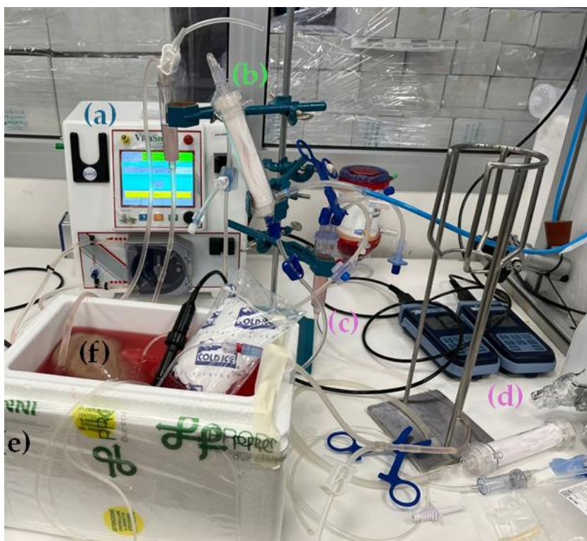
Figure 2.3.1. Perfusion setup for the kidneys: (a) perfusion machine (Bridge-to-Life®), (b) oxygenator, (c) bubble-trap chambers, (d) oxygen and temperature sensors, (e) tank containing the perfusate, (f) kidney.
