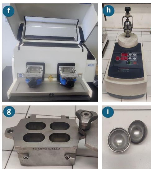
Mechanochemical instrumentations for high temperature reactions: f) MM-500 Control mixer mill, g) stainless-steel (SS) jar (4 x 10 mL), h) Fritsch Pulverisette-23, i) stainless-steel (SS) jar (10 mL) for Fritsch Pulverisette-23.
