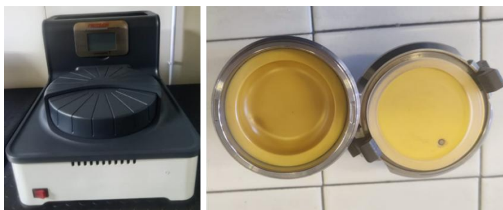
Figure 1.4. Fritsch P7-Premium planetary mill (left) and zirconia jar for planetary mill (right)
