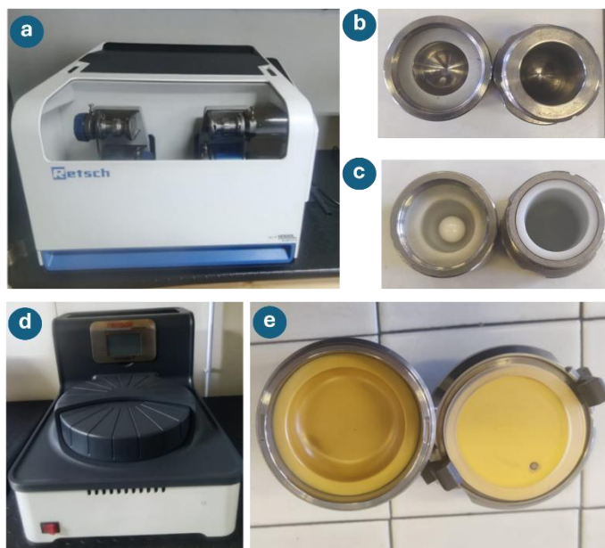
Mechanochemical instrumentations for room temperature reactions: a) MM-500 Vario mixer mill, b) stainless-steel (SS) jar (10 mL), c) zirconia jar (10 mL), d) Fritsch-P7 Premium planetary mill, e) planetary mill jar (zirconia, 20 mL).
