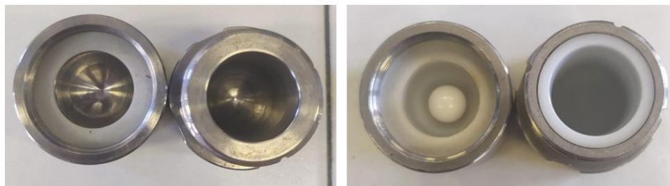
Figure 1.6. Stainless steel [SS] 10 mL ball mill jar (left) and Zirconia 10 mL ball mill jar (right)
