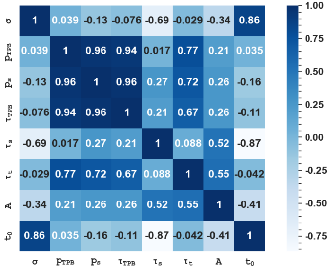
Figure 3.6: Correlation matrix of fit parameters of DarkSide-50 calculated while fitting groups of 50000 waveforms.
