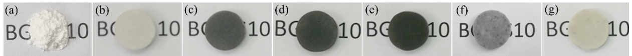
Figure 2.6: Images of (a) initial BGMS10 powder and the corresponding bulk samples produced by SPS at different T_D values: (b) 650°C, (c) 700°C, (d) 750°C, (e) 850°C, (f) 900°C, and (g) 950°C.
