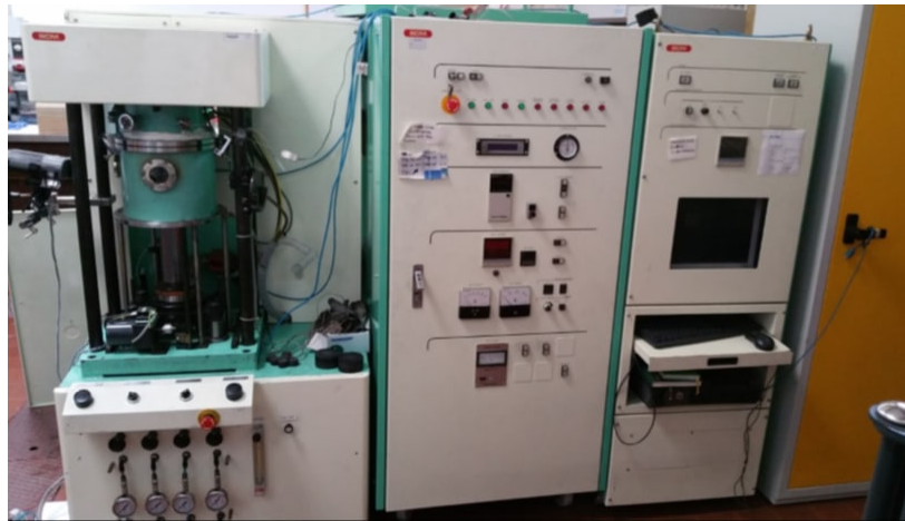
Figure 2.1: Spark Plasma Sintering equipment (model 515S) used in this work.
