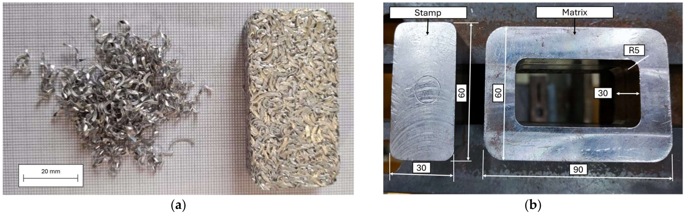
Figure 2. (a) Chips before and after cold compaction; (b) picture of the die design used for compaction (all measures in mm).
