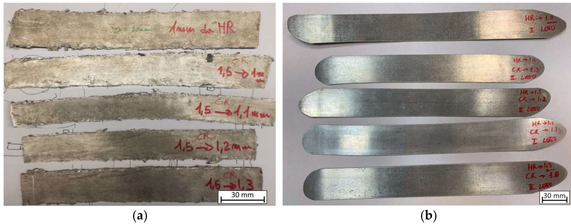
Figure 4. Hot-rolled samples following schedule in Table 2 (a) for chips and (b) for bulk materials.
