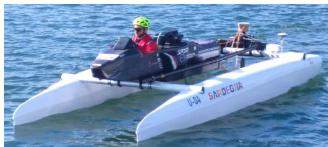
Figure 1 Typical boat Uniclass prepared by one of the crews participating in the Olbia's competition with its pilot positioned in the cockpit while preparing to start an endurance race. A rechargeable battery bank is positioned behind the cockpit.
