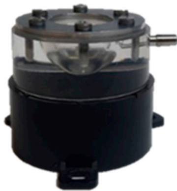
Figure 2. Mock vitreous chamber: a hollow hemisphere made of Plexiglas with 4 cc volume to simulate the vitreous chamber, closed at the top by a silicone membrane allowing trocar puncture and watertight cannula placement for infusion.
