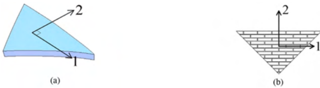
Fig. 13. Orthotropic model for masonry: definition of the two main directions (a) on the NURBS surface and (b) with reference to the masonry texture.
