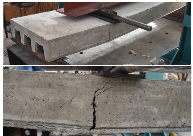
Fig. 11. Flexural crack at the end of the test.
