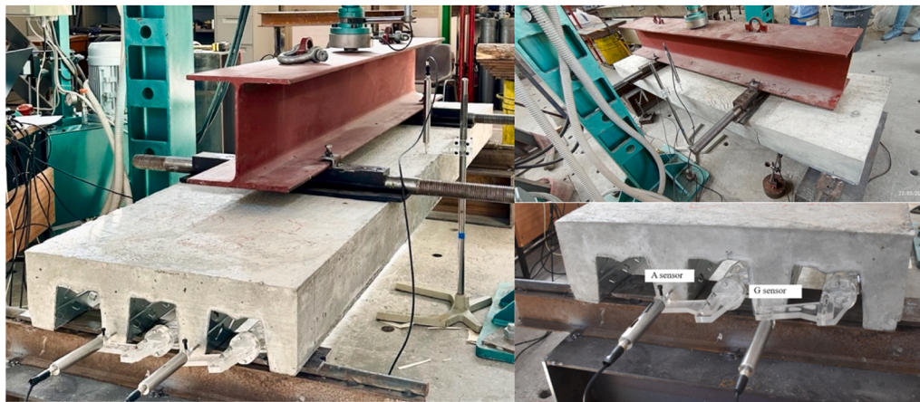
Fig. 6. Experimental set-up of the composite slab test. Top: drawings and sensors location, bottom: pictures from the experimental tests.
