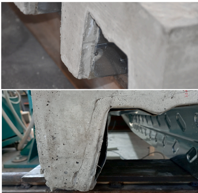
Fig. 10. Typical relative displacements of the steel sheet with respect to the concrete during the test.
