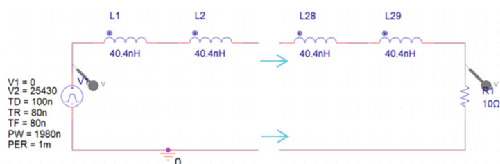
Figure 4.3.8.5: The PSpice circuit model of lumped parameter kicker system
