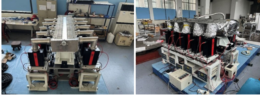
Figure 4.3.8.74: The vacuum test of half-in-vacuum Lambertson prototype for HEPS
