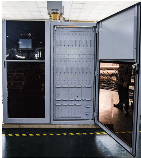
Figure 6.4.2.1: 650 MHz /75 kW solid state amplifier.
