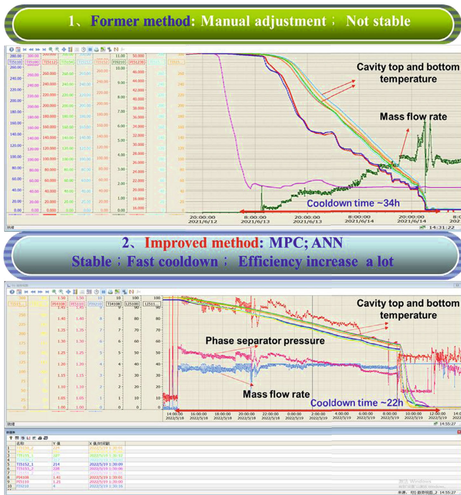
Figure 7.1.46: Environment cooldown test curves comparison between the former manual adjust method and improved cooldown method.
