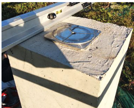
Figure 7.2.4: Auxiliary control point
