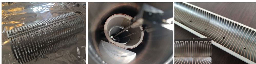
Figure 4.3.8.35: Preparation and experiment of coating with ladder pattern.
