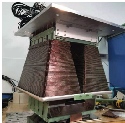
Figure 6.3.4.6: SSM pulse transformer (320 kV /380 A /4 \mu s /50 pps).
