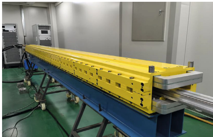
Figure 5.3.3.13: The dipole magnet with the hall probe measurement system in it.
