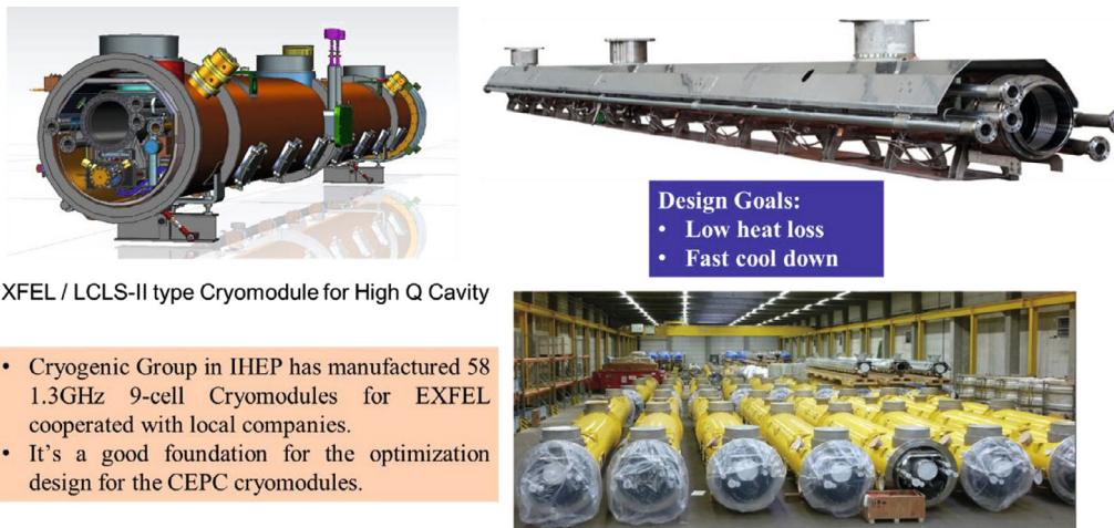
Figure 7.1.16: The 58 1.3 GHz 9-cell cryomodules manufactured by IHEP in collaboration with companies in China for the EXFEL.
