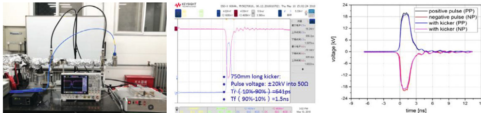
Figure 5.3.7.16: HV test of the 750 mm-long strip-line kicker prototype.
