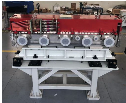
Figure 4.3.8.73: Assembly of half-in-vacuum Lambertson magnet prototype for HEPS
