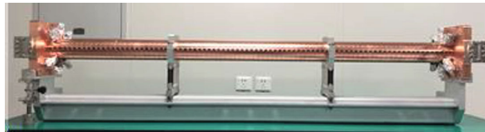
Figure 6.3.3.10: C-band accelerating structure at IHEP.
