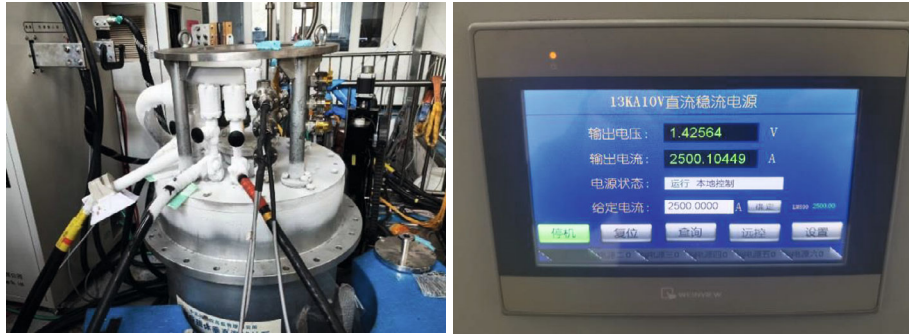
Figure 4.3.4.23: Cryogenic test of the 0.5m single aperture short model quadrupole magnet.
