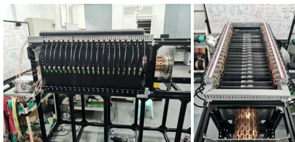
Figure 4.3.8.53: An 18-stage inductive adder prototype
