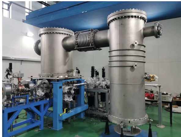
Figure A8.2.1: A photocathode DC high-voltage electron gun developed at IHEP.
