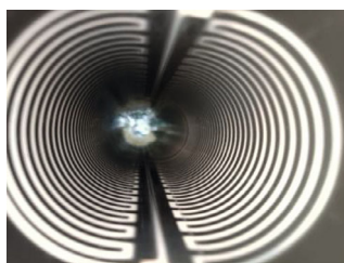
Figure 4.3.8.36: Ladder-shaped coating on racetrack-shaped ceramic vacuum chamber.
