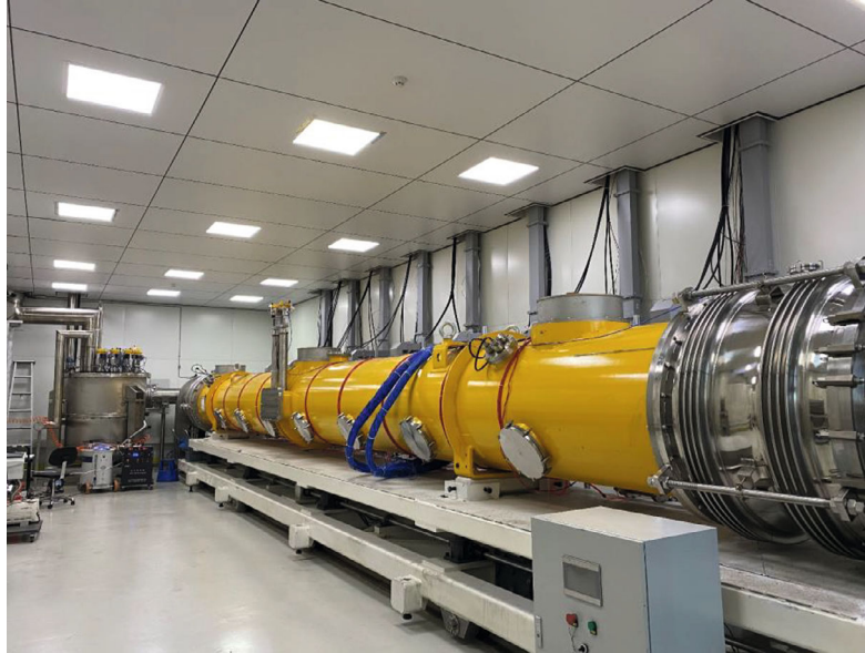
Figure 7.1.26: Assembly photo of the 1.3 GHz cryomodule.
