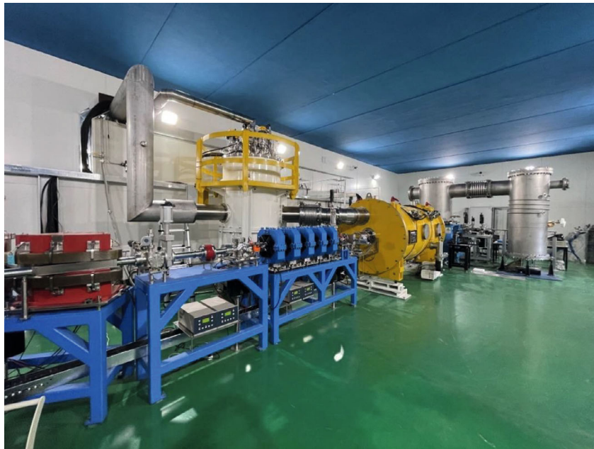
Figure 7.1.27: Prototype cryomodule with two 2-cell 650 MHz superconducting cavities on the PAPS beam test stand.
