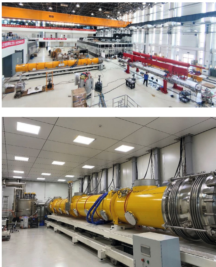
Figure 5.3.1.2: Assembly and horizontal test of the 1.3 GHz cryomodule
