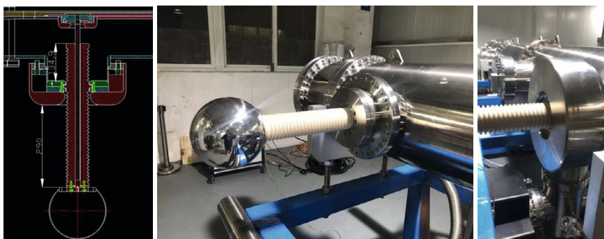
Figure 4.3.11.21: Improved feedthrough of the electrostatic separator.
