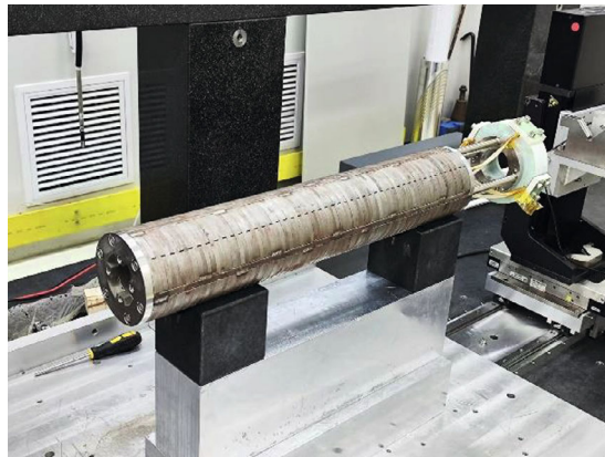
Figure 4.3.4.22: A 0.5m single aperture short model quadrupole magnet.
