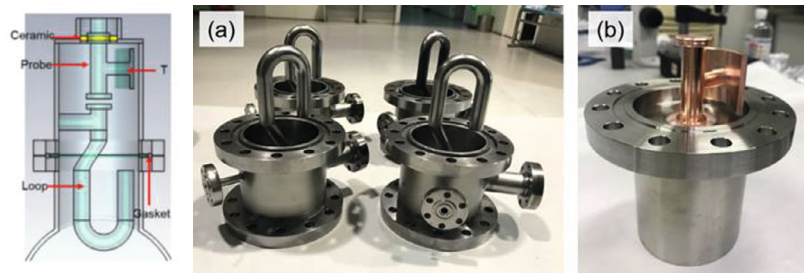
Figure 4.3.1.9: Double notch HOM coupler with two parts: (a) niobium hook part (b) copper probe part
