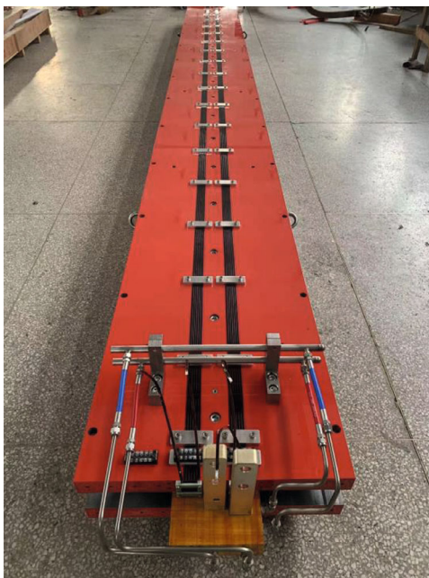
Fig.4.3.3.11: The 5.7 m long dual-aperture dipole magnet prototype.
