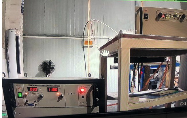
Figure 4.3.11.21: High voltage test of the electrostatic separator.
