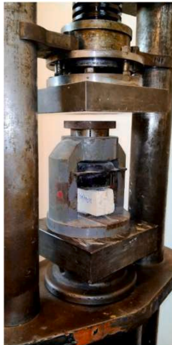
Fig. 11. Compression strength test: sample M1F0.5(30) M1S2.
