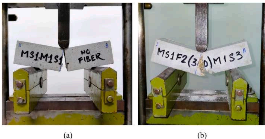
Fig. 14. Samples (a) MS1M1S1 without fiber and (b) MS1F2(30)M1S3 with 2% fiber (30 mm) with respect to dry mortar mass.
