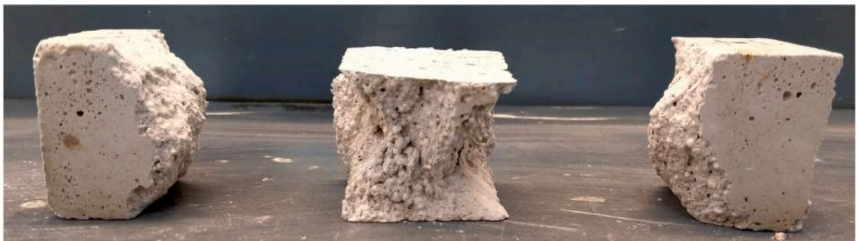
Fig. 25. Thermal mortar sample M1M2S2 without fiber, after compression failure.
