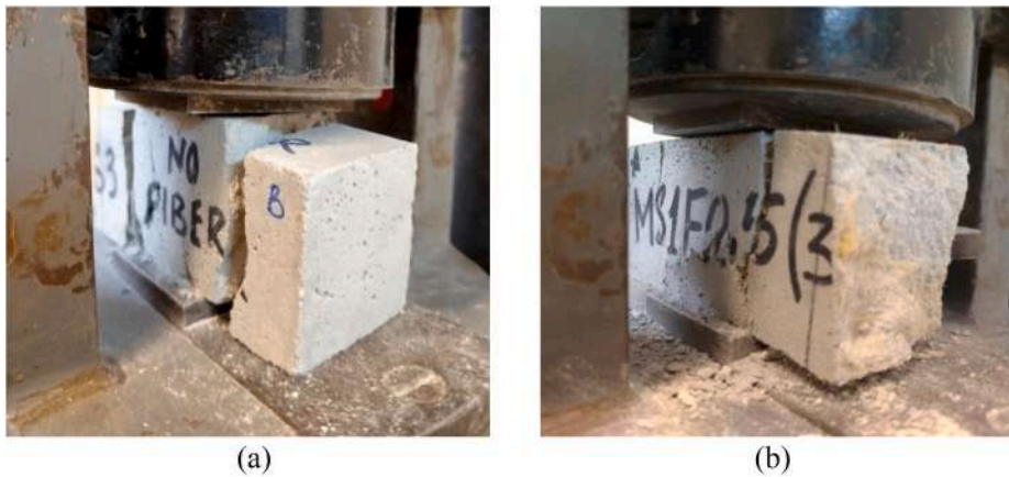
Fig. 24. Structural mortar samples ultimate compression rupture (a) MS3M1S3 without fiber and (b) MS1F0.5(30)M2S3 with 0.5% jute fiber (30 mm) with respect to the dry mortar mass.
