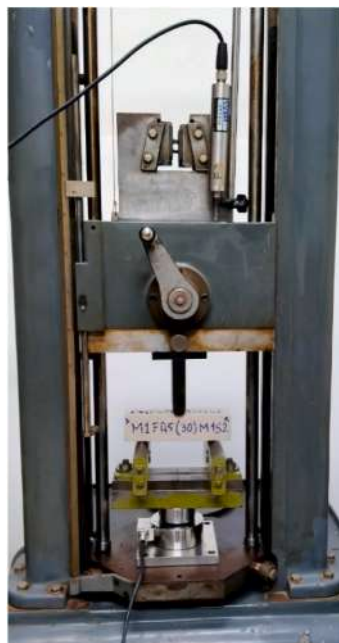
Fig. 9. Flexural strength Test: Sample M1F0.5(30) M1S2.
