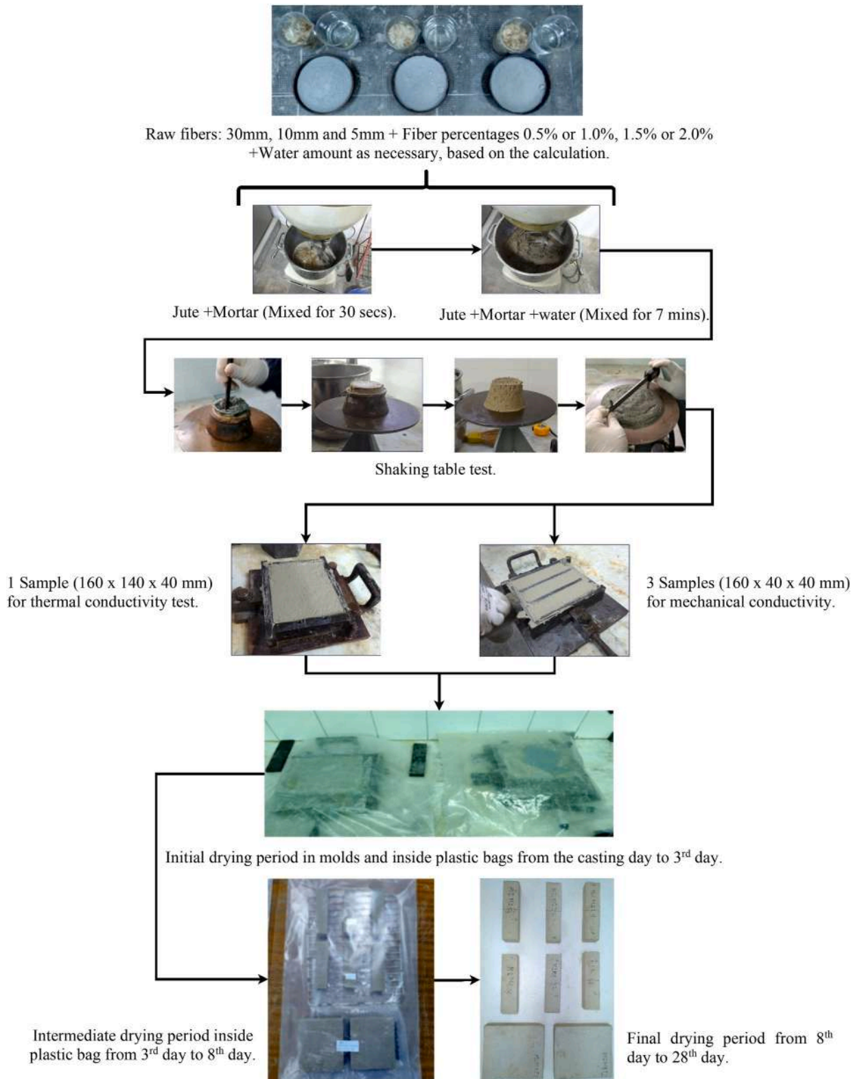
Fig. 4. Jute fiber composite mortar preparation.
