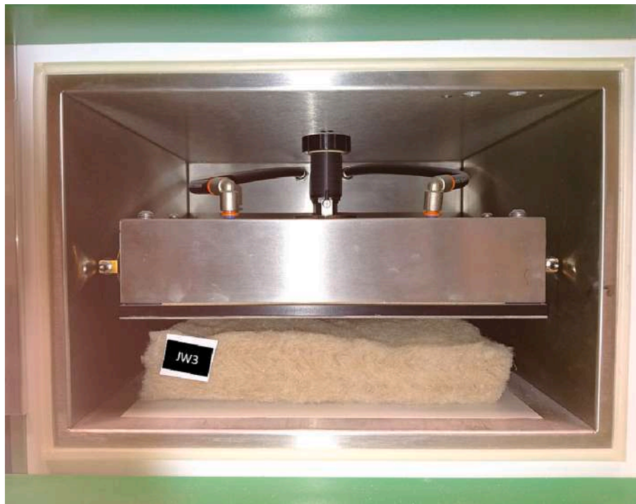
Fig. 8. Sample JW3 with 250 × 250 mm 2 inside the TAURUS measuring chamber.
