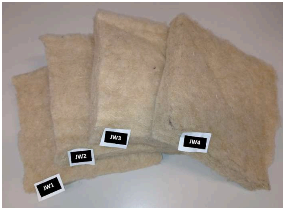
Fig. 2. Insulation panel made of recycled jute and wool fiber.
