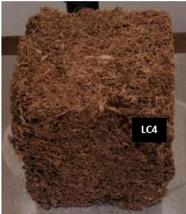
Fig. 6. Insulation materials: Loofah fiber and clay used as binding material.
