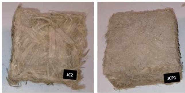
Fig. 4. (a) Insulation material: Jute fiber and clay used as binding material, (b) Insulation material: jute fiber and clay used as binding and plaster materials.
