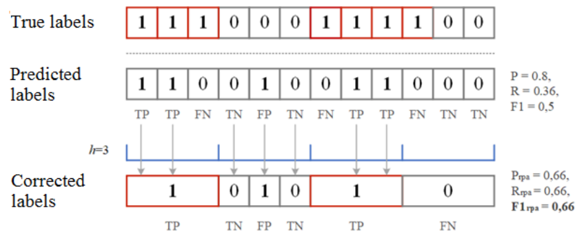
Figure 5. True, predicted, and corrected labels in case of the RPA approach to the metrics calculation.
