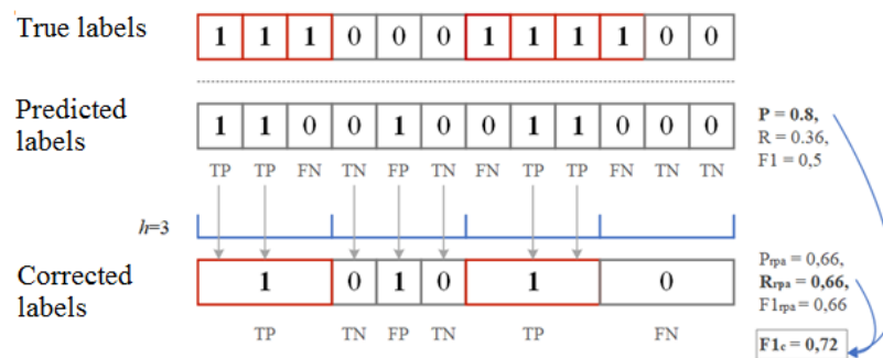
Figure 6. True, predicted, and corrected labels in case of the composite F1 score approach to the metrics calculation.
