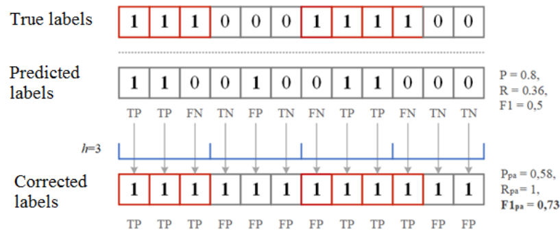
Figure 4. True, corrected, and predicted labels in case of the PA approach to metrics calculation.
