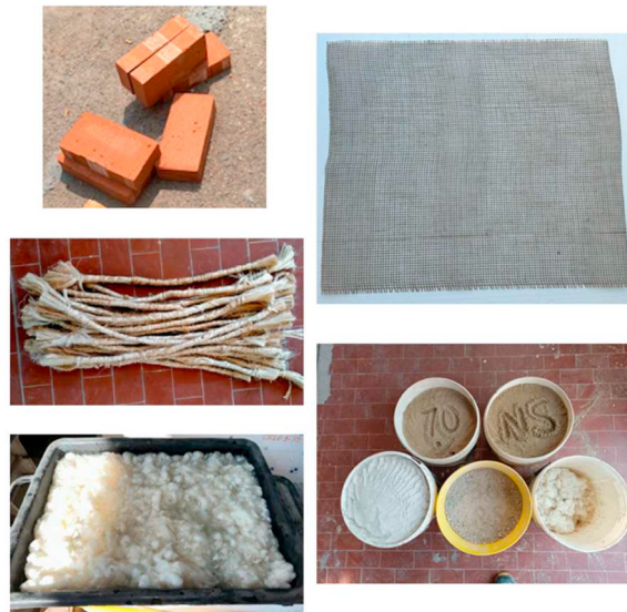
Fig. 1: Materials used for the wall preparation. The strengthening configuration included jute diatons with a constant density of approximately 2.78 diatons/m 2
