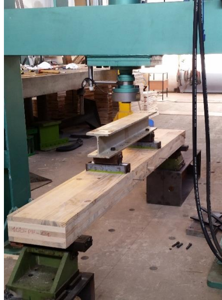
Fig. 9. Laboratory set-up of loading configuration for bending test of 100-PF CLT specimens.
