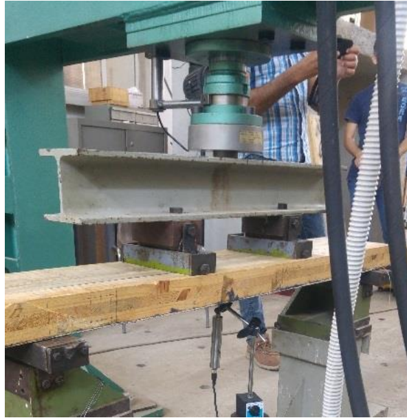
Fig. 5. Loading set-up for bending test of 60-PF CLT specimens.
