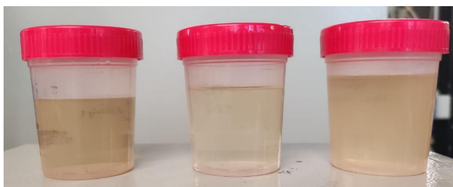
Figure S4.2 – From left to right, fresh swine denitrified effluent, anolyte and catholyte by the end of a precipitation test in the batch electrochemical system.
