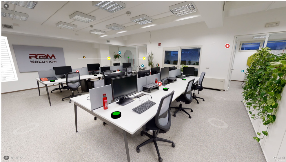
Fig. 4. Occupation sensor widgets inside of the Digital Twin. At the time of the screenshot, the three seats in front of the respective workstations were free.
