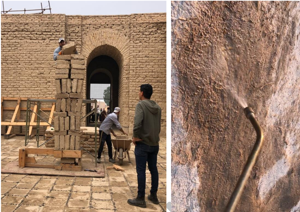
Photo 8. Compression tests on adobe and water resistance test on earth-lime plasters. Credits: M. Achenza
