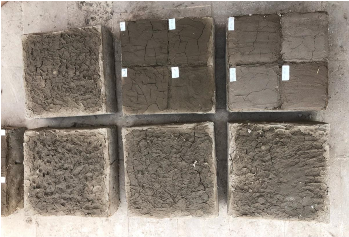
Photo 6. Tests and samples for plasters and mortar. Credits: M. Achenza
