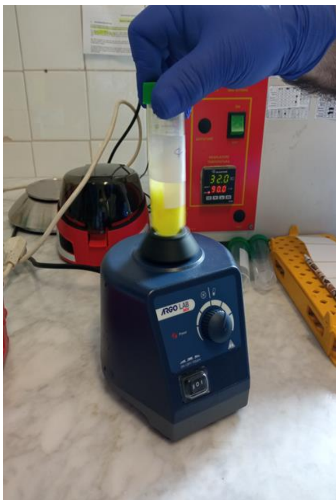
Fig. 34. Mixing EVOO with hydrogen peroxide, before separating the oil fraction.
